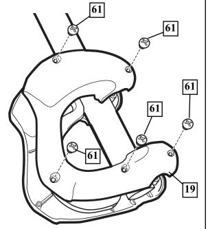
Attach adjustment tube to lower elevator tubes using bolt spacers and nut as shown.
